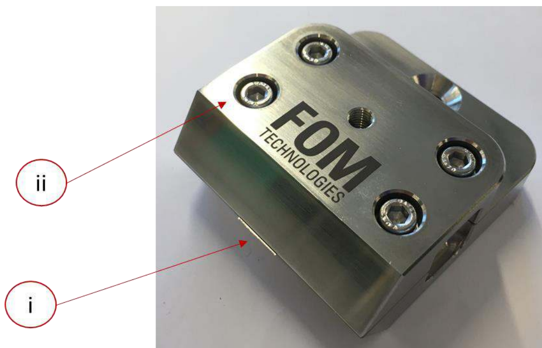
Figure 2.3. Fully assembled slot die head. (i) The shim tooth visibly protrudes from the coating lip of the slot die head. (ii) The securing bolts (x4) are inserted to lock all components together.
